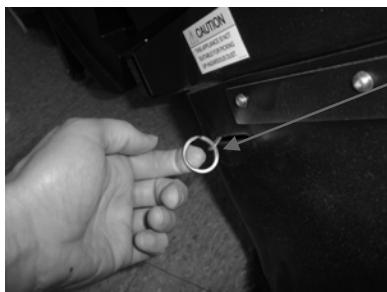
A thin film of lithium grease may be applied on the lead-in chamfers of the Rubber Mounts to allow for easier ramp installation. Wipe off all excess grease.
