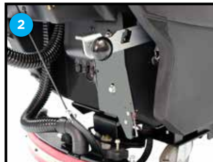
Medium down pressure when lever is hooked in mid-position
