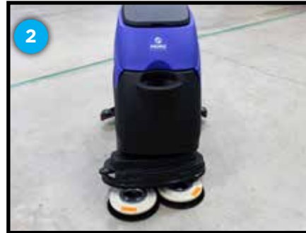
Position scrub head over pad drivers or brushes
