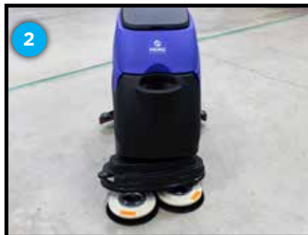
Cleaning tools released by auto on/off feature
