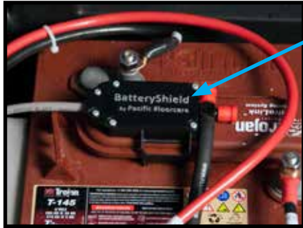
BatteryShield optical sensor on Trojan battery
