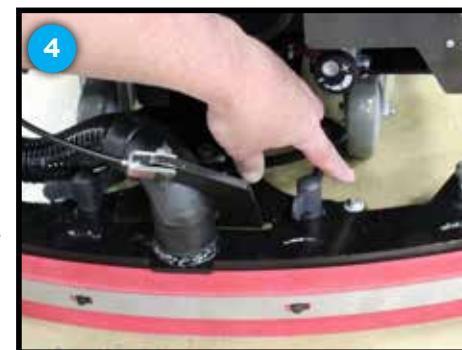
Button screw to raise and lower squeegee assembly wheels
