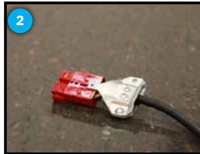
Anderson connector located on charger cable
