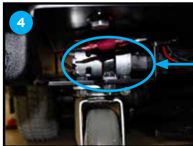
Check solution pump (circled) for vibration from rear of unit
