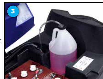
3 Chemical bottle connected properly to chemical injection system
