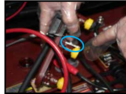
HydroLink battery cap light pipe circled above
