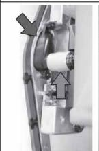
5. Verify the tightness of the drain hose and drain plug.
