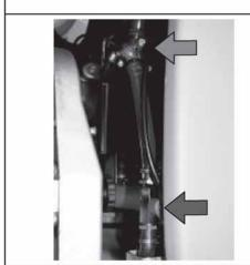
Make sure, that with the valve open, the solution arrives continuously on the floor.
