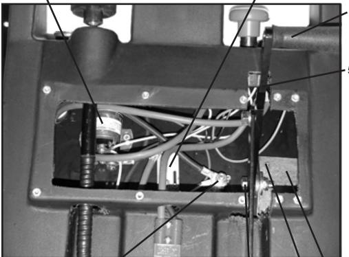
911610 Cable Stud (1) 962066 Screw-8-32x3/4 PHP (2) W440D Nut-8-32 Hex w/Nyloc (2) 525112 Bracket-Lift Handle (1)
