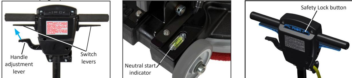
Once you have the handle height set to your preference and you are in the operators position, look to the right on the base of the machine. You will see the neutral start indicator which indicates with the base of the machine is level by aligning the bubble in between the two lines. Press in on the Safety Lock button with your thumbs and start the machine by depressing either the left, right or preferably both switch levers.
