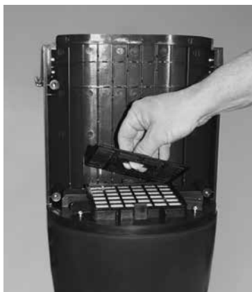
Figure 6 - Removing HEPA filter
