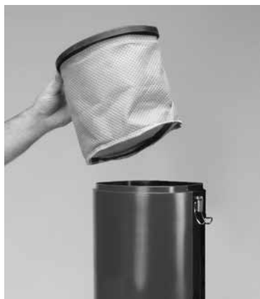
Figure 5 - Removing cloth bag
