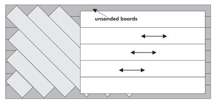
Sand and blend edges in with main floor area.
