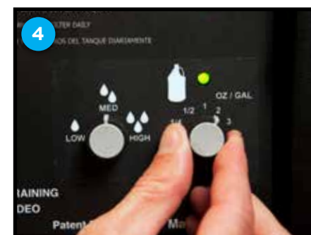
Chemical injection chemical mix ratio dial being set
