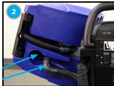
Upper elbow of recovery hose and recovery tank orifice
