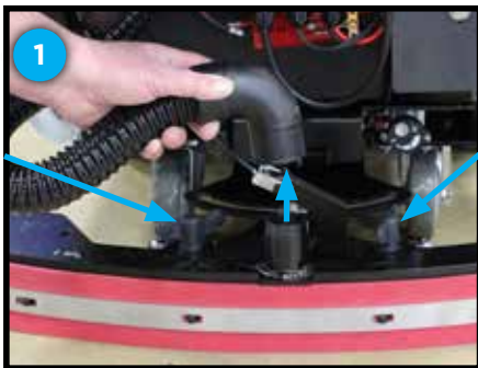
Loosen the two easy-grip knobs and detach recovery hose to lift away the squeegee assembly
