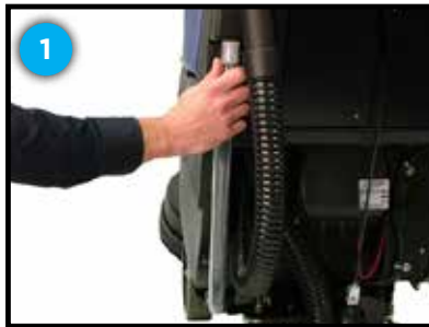
Check sight gage hose for solution level
