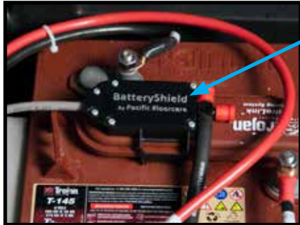
BatteryShield optical sensor on Trojan battery
