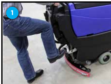
Lowering scrub head using foot pedal
