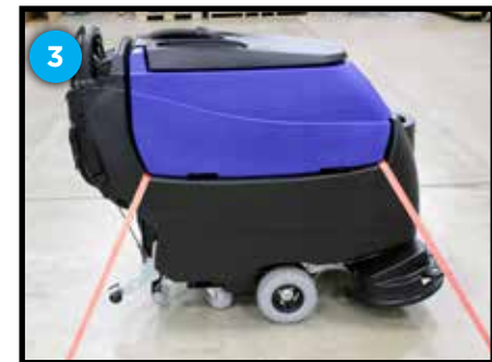
Tie down locations between recovery tank and solution tank
