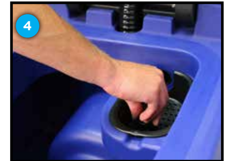
Press the TTS holder and bromine puck back into the debris tray
