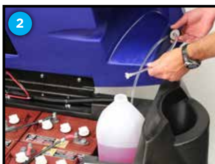
1-gallon chemical bottle in holder, preparing to insert leader hose
