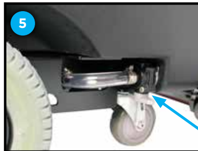
Check to make sure that the ball valve is open
