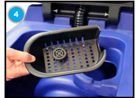
Empty debris tray and clean out
