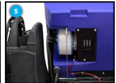
Remove the HEPA filter and visually inspect it. Replace if necessary
