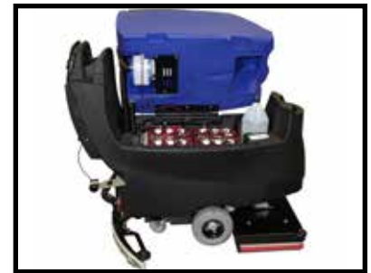
Recovery tank shown in fully open position
