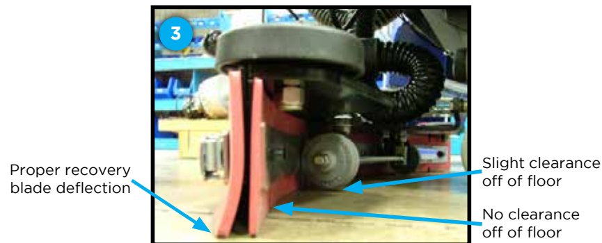
Close up of squeegee assembly and blade deflection
