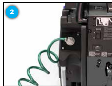
Auto-off solution fill system connected to scrubber
