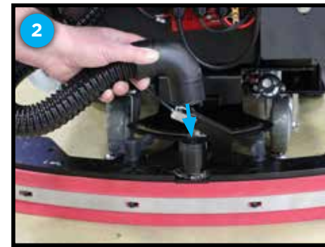
After aligning assembly, tighten the easy-grip knobs and attach the recovery hose
