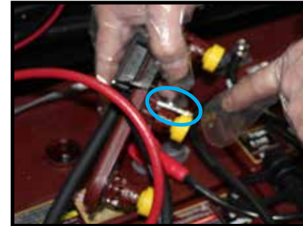
HydroLink battery cap light pipe circled above
