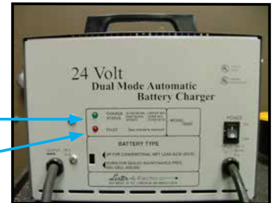
Charging indication LEDs (charger appearance may vary)
