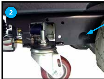
Tie down location on main frame
