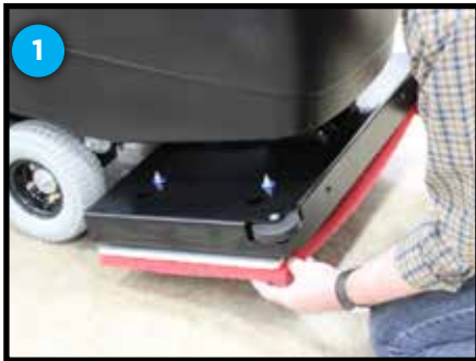
Align the front corners of the pad and press to adhere
