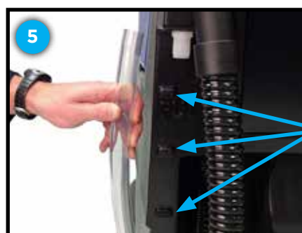
Sight gage hose released from press fitting
