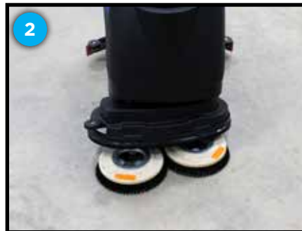
Cleaning tool released by auto on/off feature (S-24XM)
