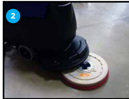
Position scrub head over pad driver(s) or brush(es) (S-20 shown)
