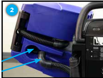
Upper elbow of recovery hose and recovery tank orifice
