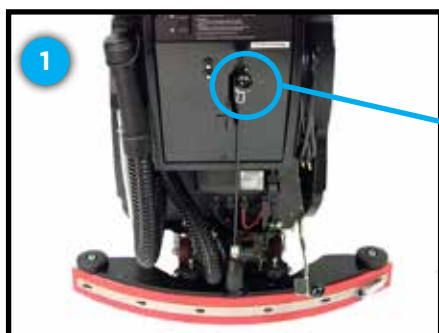
Squeegee assembly in transport/storage position
