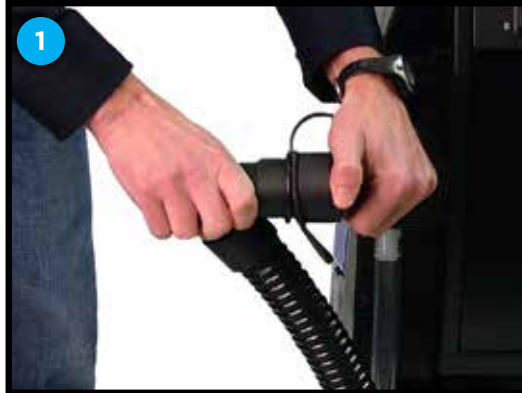
Check for clog in the restriction collar
