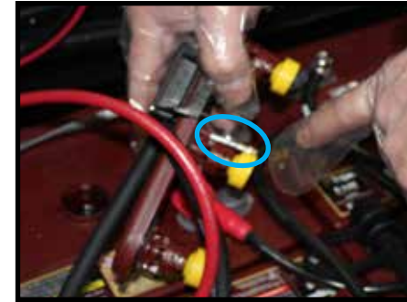
HydroLink battery cap light pipe circled above
