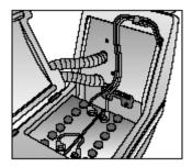
**NOTE:** Never leave the batteries completely discharged, not even if the machine is not being used. When recharging, first empty the recovery tank and then open the recovery tank. Check the level of battery electrolyte every 20 recharges. Top up with distilled water as necessary. (WET LEAD ACID ONLY)
