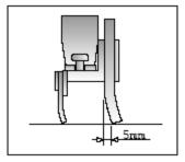
The rear rubber, during operation, must be slightly and uniformly bent back about 5 mm. along its entire length. It may be necessary, to increase curvature of the rubber in its central section, to slope the squeegee body backwards. This is done by rotating adjustment unit (1) counter-clockwise. To increase curvature on the outside sections of the rubber just rotate adjustment unit (1) clockwise.
