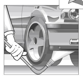
Always aim the underbody lance. Note when using an angled underbody lance, like for example lance No. 41.075 1, that there is a certain amount of torque in the recoil. (See also notice on page 2)
