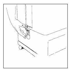
2. Fill the solution tank with cold or warm water through the filling hole. Add non-foaming chemical to the solution tank, diluting it according to the manufacturers specifications.
