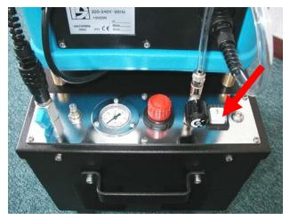
9. Switch on the vacuum motor.
