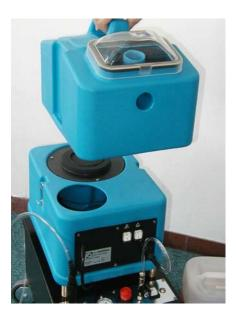
4. Add warm water into the solution tank. Add chemical in to the solution tank according to the dilution rate suggested by the manufacturer.
