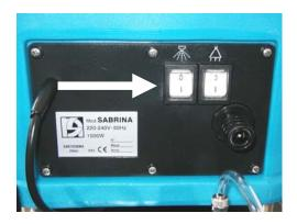
8. Switch the air compressor on by moving the switch to the position "I". The compressor switch is located on the foam regulation control panel. The compressor will run until full tank pressure is reached (Approx. 1 minute). After this, the compressor motor will only turn on to recharge the tank.
