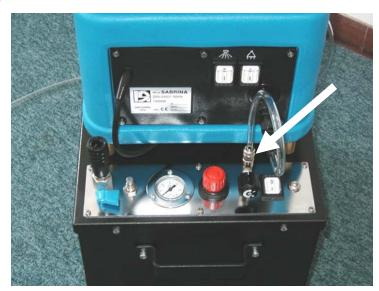
2. Check that the valve at the foam outlet is closed. Connect the solution hose to the foam outlet and then open the foam outlet valve.
