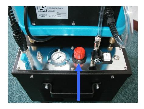
Before making any adjustments, you must wait for the compressor to come up to full pressure.
