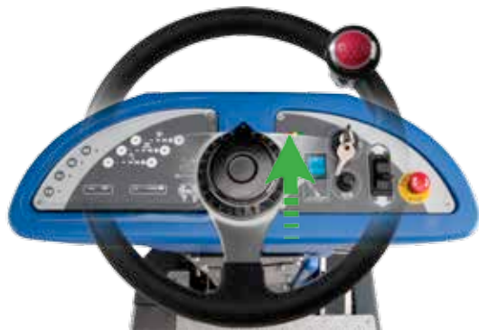
Showing location of Viewing panel for charging-light sequence.
