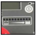
Batteries should be recharged every three months. Charge fully the day before you start using the machine again.
