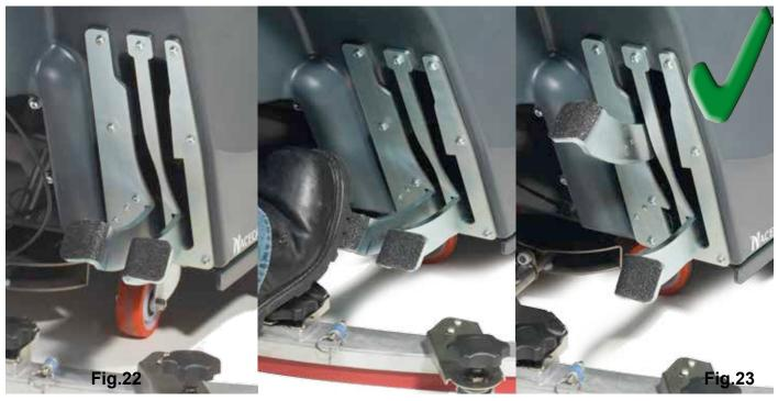
The control for lowering the brush deck can be found to the rear right of the machine (Fig.22). Lower the brush deck by moving the left hand release lever to the upper position (see Fig.23).
