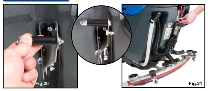
After preparing the floor (see previous section), we are now ready to set the controls to suit the cleaning conditions. Before any settings can be applied, ensure the brush deck is lowered (see Fig.23). Move the floor-tool lever (see Fig.20), to it's lower position (see Fig.21).
