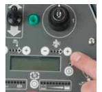
Set automatic Chemical Dosing Mix as required, depending on floor type and level of soiling.
