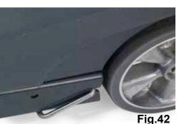
Swing to the disengaged position (see Fig.42).
