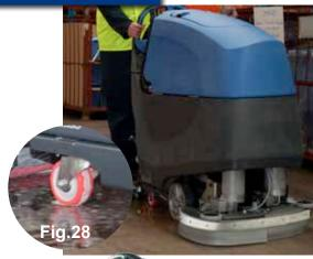
Vacuum pick-up, water-flow and chemical-dose will turn on automatically and the machine will move forward.
