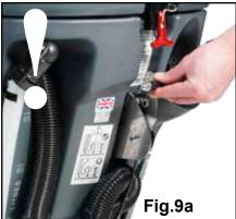
Lower the floor-tool arm by moving the release lever to the lower position (Fig.7). Push floor-tool onto the holder and secure with the easy-fit securing pin (Fig.8). Push waste collection pipe onto the floor-tool; ensure a tight fit (Fig.9). Note: Raise floor-tool again before driving to the cleaning area (Fig.9a).
