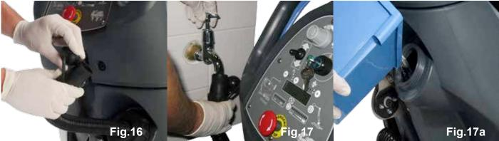
To fill the clean-water tank, extend the hose located to the rear of the machine in the centre of the removable filler cap, see (Fig.14). Pull out hose, (Fig.15). Open the stopper (Fig.16) and place hose under water tap, or use a hose to commence filling, (Fig.17).
