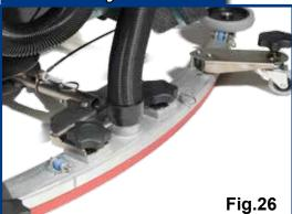
The floor-tool design incorporates a breakaway feature.
