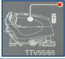
When the waste-water tank becomes full, a red warning light will illuminate on the operator control panel (as illustrated).
