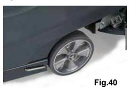
The motor brake is located on the left side of the machine near the rear wheel (see Fig.40).
