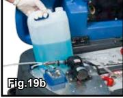
To fill the chemical-dosing bottle, first make sure the top waste tank is fully drained then, lift up the waste-water tank (Fig.18), remove the dosing bottle, unscrew the bottle cap (Fig.19) and fill with appropriate cleaning chemical, or fit your own chemical container, reusing the original Numatic container cap 1.5 inch / 1.65 inch (Fig 19a). Refit dosing bottle (Fig.19b) and replace bottle cap, and carefully lower waste-water tank.
