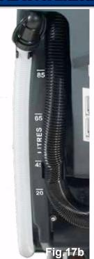
The water level in the clean water tank can be measured using the scale on the rear of the machine (Fig.17b).
