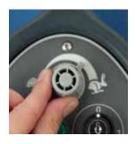
Set desired traction Speed as required, depending on floor type and level of soiling.
