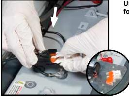
If the machine will be standing unused for a period of 30 days or more, then batteries must be fully charged and battery fuses removed using the Maxi fuse-puller provided, prior to this period.
