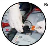
Recharge the machine fully after its last use. Do not leave the machine in a discharged state.
