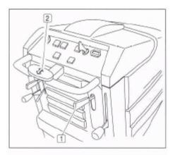
Immediately apply emergency brake (11 on the right side of the machine whenever problems arise during operation. This control stops forward movement by the machine. To start to work again, after solving the problem, just raise lever (1) and push directional lever (2) forward.
