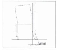
The rear rubber, during operation, must be slightly and uniformly bent back about 5 mm. along its entire length. It may be necessary, to increase curvature of the rubber in its central section, to slope the squeegee body backwards. This is done by rotating adjustment unit (2, fig. 31 counterclockwise. To increase curvature on the outside sections of the rubber just rotate adjustment unit (2, fig. 3) clockwise.
