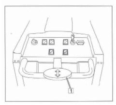
The machine will start to move when directional lever (1) is pushed forward. Check, during the first few meters of wash, that brush pressure is adequate bee "BRUSH PRESSURE below), that the amount of water is sufficient and that the squeegee dries the floor perfectly.
