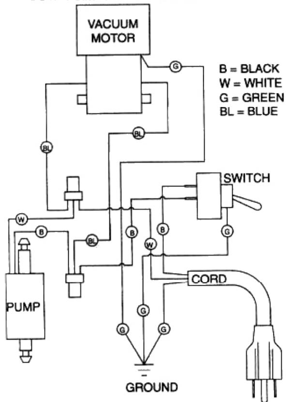
PUMP + VAC TURN ON SEPARATE OR TOGETHER
