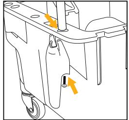
Or follow included instructions to attach OHORN screwing directly into Handle
