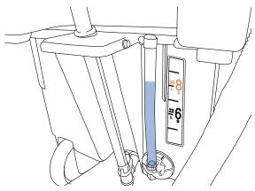
CAUTION: Before filling with solution, ensure the spigot is in the "OFF" position.
