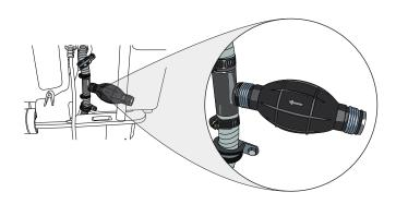
**To prime the pump:** Squeeze Primer Bulb 10 times prior to initial startup, or if pump has been run dry for any length of time.
