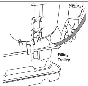
Note the location of the Sight Gauge on the back of the Trolley-Bucket.
