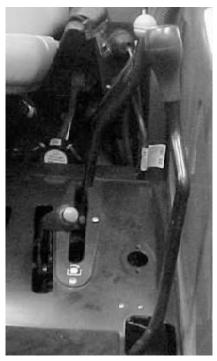
If the squeegee is in the down position and the tractor shift lever is moved into the reverse position, the squeegee will automatically raise and the solution vacuum will turn off. Once the shift lever is returned to the forward or neutral position, the squeegee will automatically lower and the solution vacuum will be turned on
