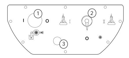
Solution Pump Switch (1): turns the solution pump on/off
